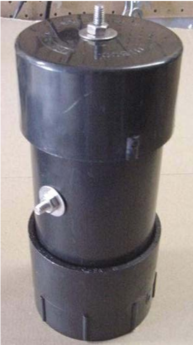
This is the finished e-cell shown here upside down. Assemble the unit using ABS glue.
