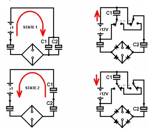
Here, two capacitors are used instead of two batteries. If the size of the capacitors is matched to the switching
