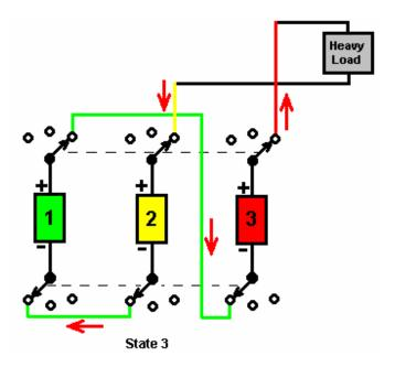
The challenge then, is to construct this using solid-state electronics and so produce a switching system with no moving parts.
