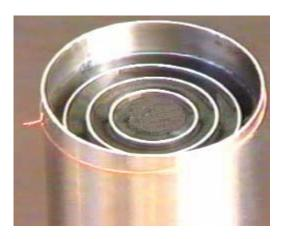
The picture above shows the general construction of a cell of this type although, unlike the description below, this one does not have the lip which is used for attaching the lid. It is included here just as a general illustration of how the cylinders are positioned relative to each other.
