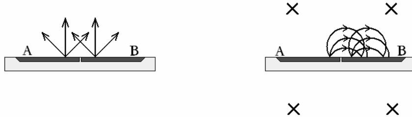
(a) Electrons ejected into a zero-field space (b) Electrons ejected into a magnetic field
