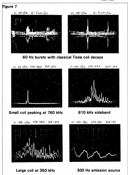
powered normally, the large Tesla coil resonates somewhere around 330 kilohertz.
