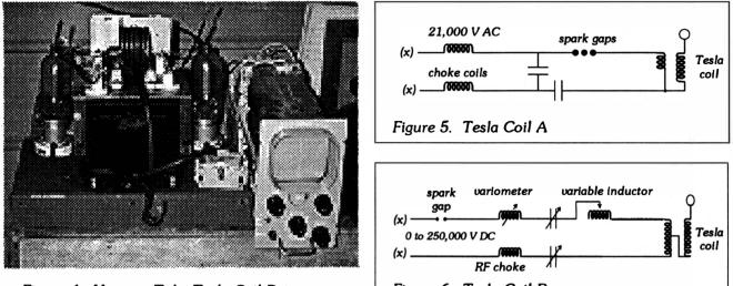
Figure 4. Vacuum Tube Tesla Coil Drive
