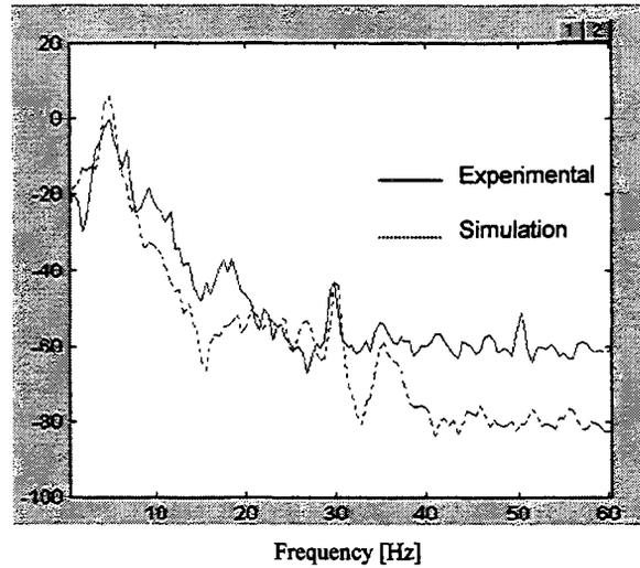
Fig. 15 Third test series PSD [dB] – Case (C) experimental and simulation results.
