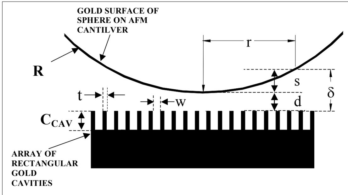
**Figure 6.** Distance definitions, illustrating actual cavity depth ( $C_{CAV}$ ), individual cavity width ( $w$ ), cavity wall thickness ( $t$ ), separation distance ( $d$ ), local sag ( $s$ ), and local separation distance ( $\delta$ ).
