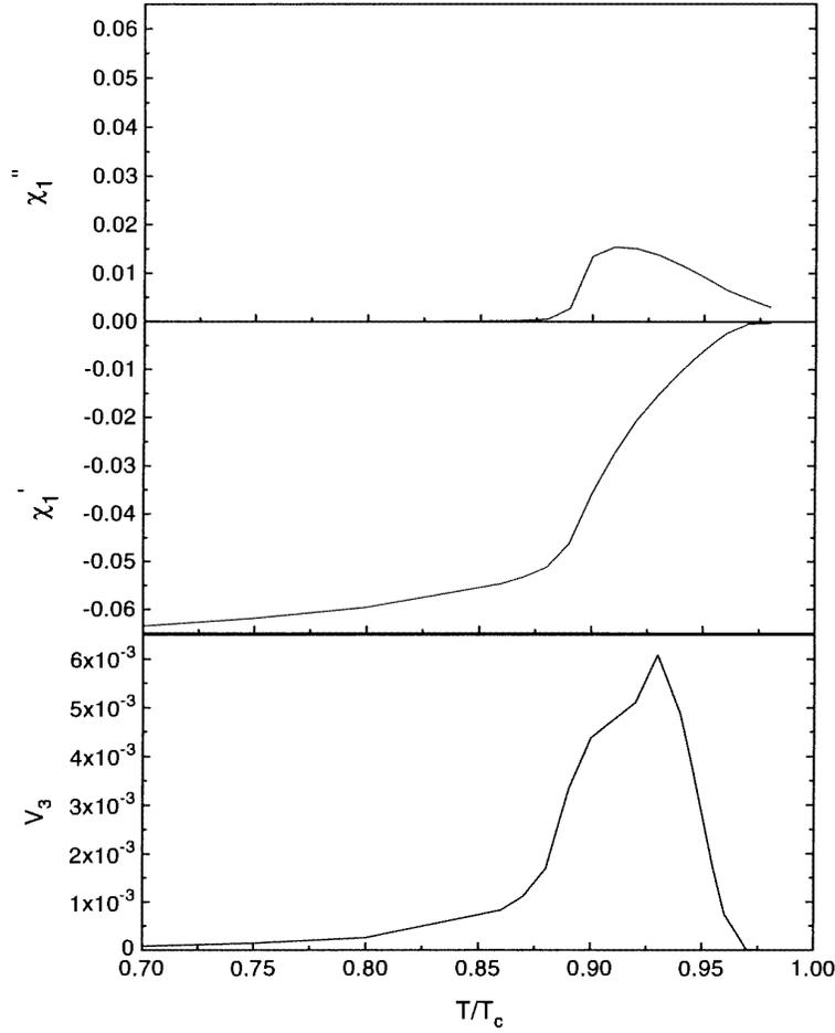
**Figure 2.** Temperature dependences of  $\chi_1''$ ,  $\chi_1'$ , and  $V_3$ .
