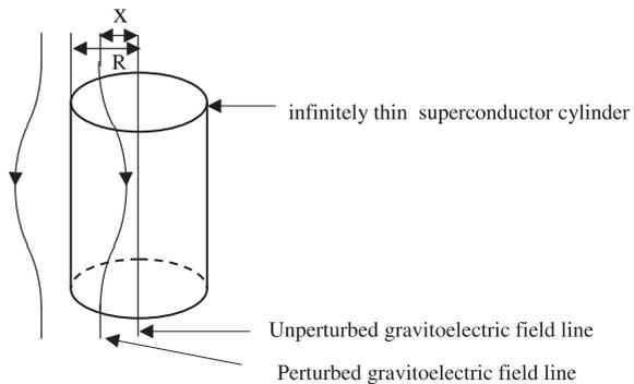
Fig. 1. Thin superconducting cylinder in a gravitoelectric field.
