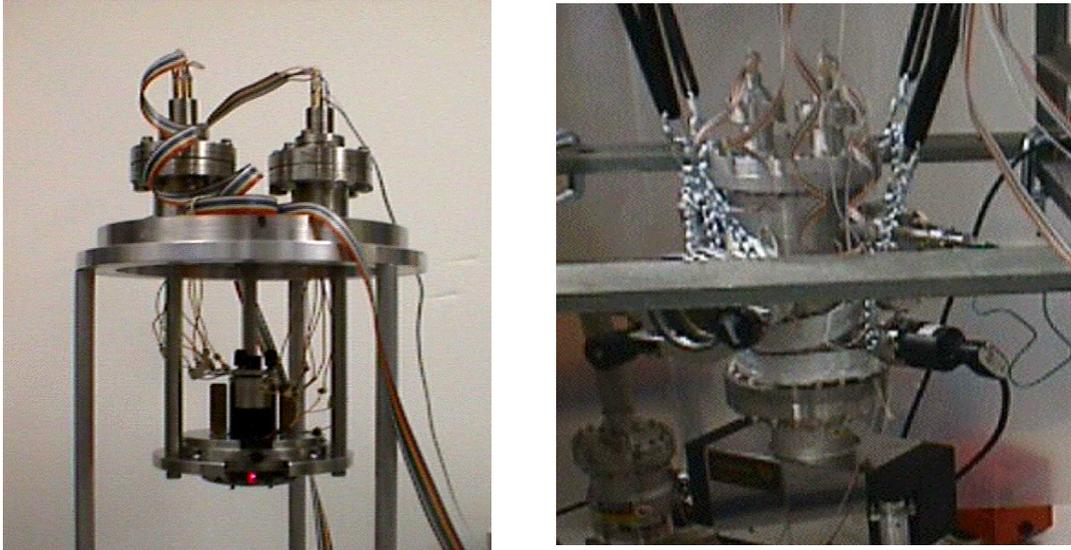
**Figure 3.** (a) shows the AFM stage below the vacuum flange, connected to the vacuum feedthroughs above. (b) shows the AFM mounted inside a small, stainless steel, vacuum chamber supported by elastic cords to reduce vibration.
