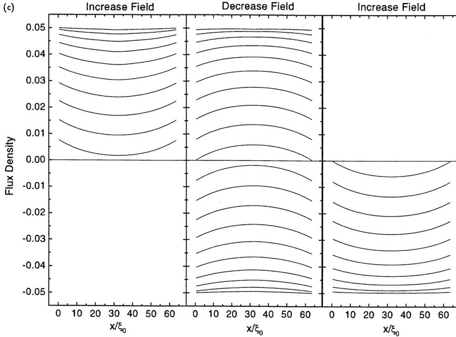
**Figure 3.** (Continued) Time variations of profiles of the  $z$ -component of the local magnetic flux density,  $b_z$ , in units of  $H_{c2}(0)$  along the  $x$ -axis at  $y = 32\xi_0$  for  $T/T_c = 0.8$  (a),  $0.91$  (b), and  $0.97$  (c). Time goes from the left-hand column to the right-hand one for one cycle of the ac field.
