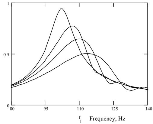
Figure 3. Measured NMR lines (left) and calculated (0,12,25,50 cm/s) for zero E-field and flows from 0 - 50 cm/s.
