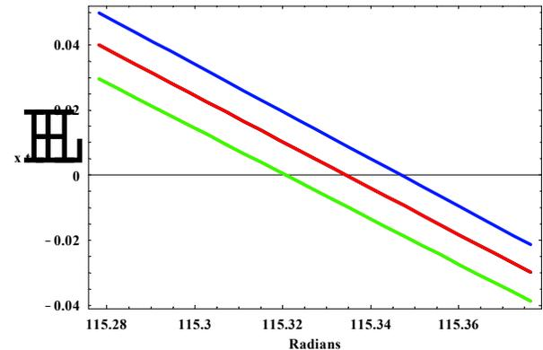
Figure 2. Response phase shifts of the system to variable mass. The central line is the system response with  $\mu_0=0$ . The other two lines represent  $\mu_0=0.001$  with  $\phi_m=-\pi/2$  (low), and  $\phi_m=+\pi/2$  (high). The phase shifts shown are about  $\pm 0.04$  radians= $\pm 2.3$  degrees.
