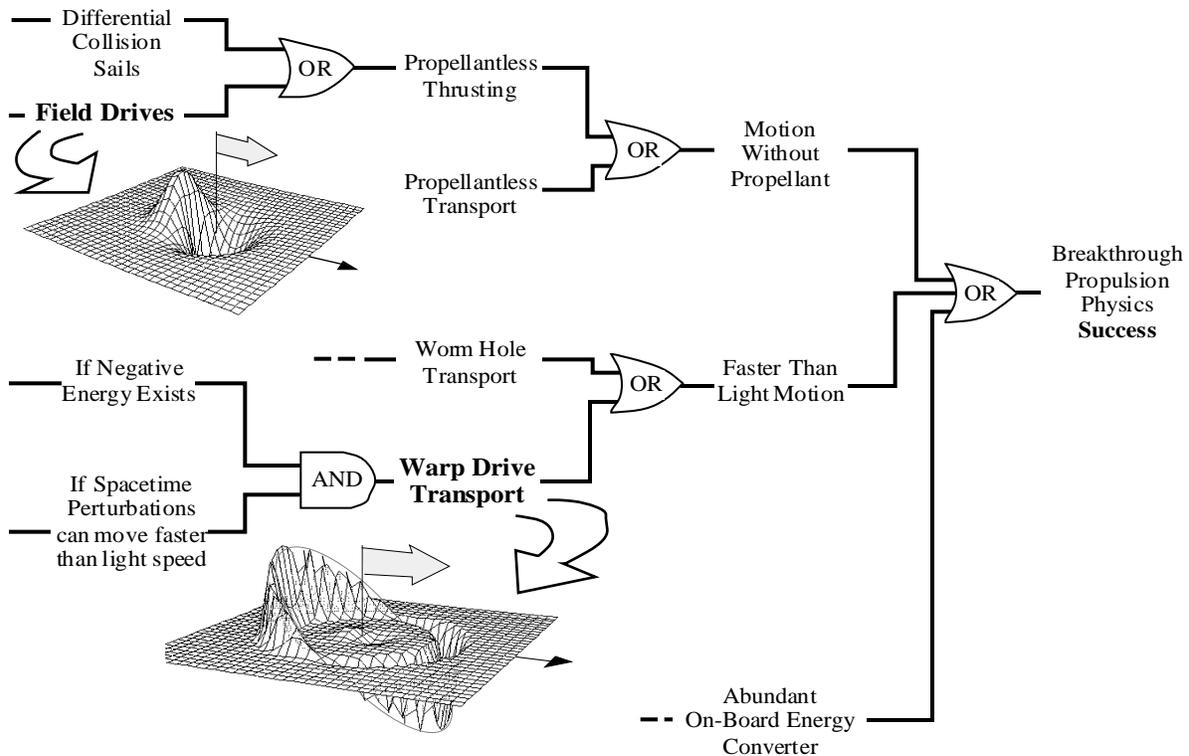
FIGURE 1. Illustrative Example of a Traceability Tree.
