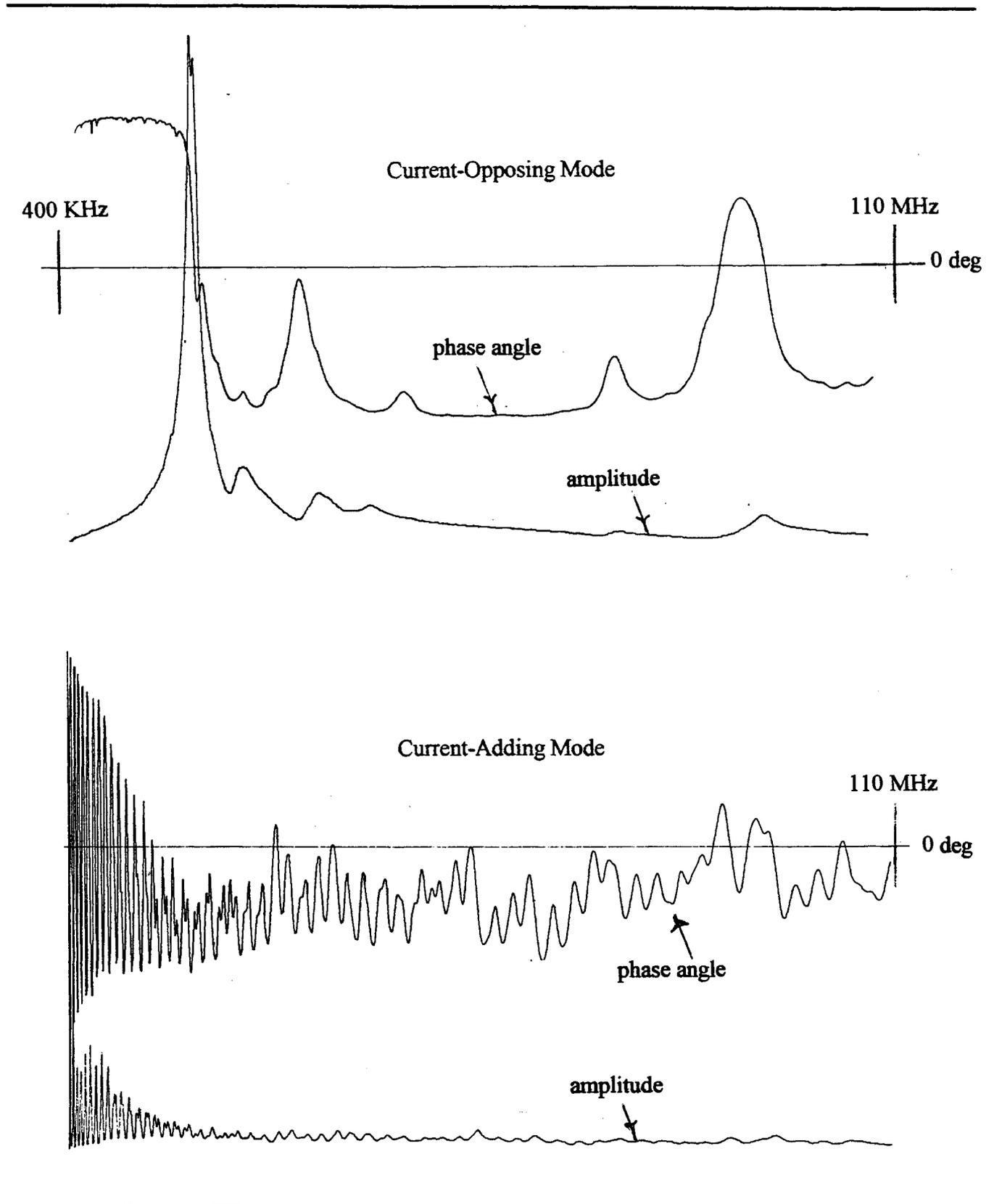
Fig. 9 – Resonances for Large Diameter Toroid
