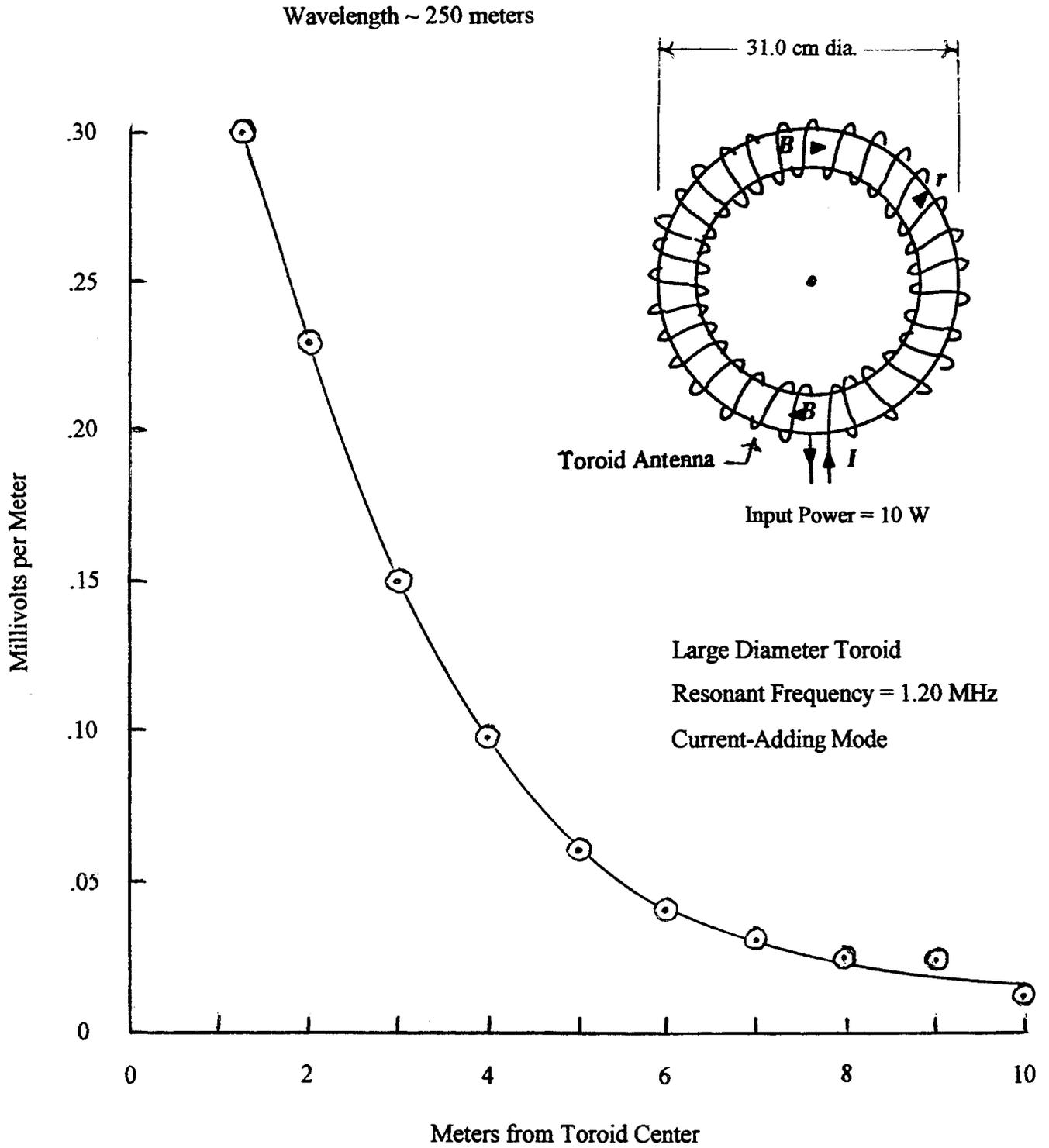
Fig. 12 - Attenuation of Toroid Signal with Range
