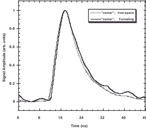
**Fig. 3:** A measure of the pulse broadening due to tunneling through the 1DPC. The two pulses have propagated along the same path (“center”); one in the free-space and the other through the 1DPC.
