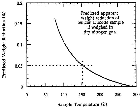
Fig. 2. Prediction of the percentage reduction in apparent sample weight of an  $\text{SiO}_2$  sample compared with its apparent weight at 290 K. The data assumes that the sample is weighed in dry nitrogen gas at atmospheric pressure, but the results are likely to be similar for dry air.
