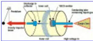
*Reported operation of high-power gravity device: the YBCO emitter is cooled to superconducting conditions and the inner electric coil produces a magnetic field inside it. A very high voltage pulse is input to the emitter which then discharges to the collector. The discharge is guided and contained by the magnetic field in the outer coil*
