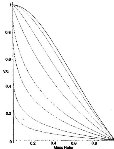
Figure 3: These plots indicate the mass-energy ratio  $M(t)/M(0)$  required to reach a relativistic speed ratio  $V/c$  in the absence of any gravitational field. Each curve has a definite ejection speed ratio  $u_0/c$  relative to the propulsion system. These are  $1/20, 1/10, 1/5, 3/10, 1/2, 7/10$  and  $9/10$  in order starting from the bottom of the plot. The advantage of relativistic mass-energy ejection is apparent from these curves.
