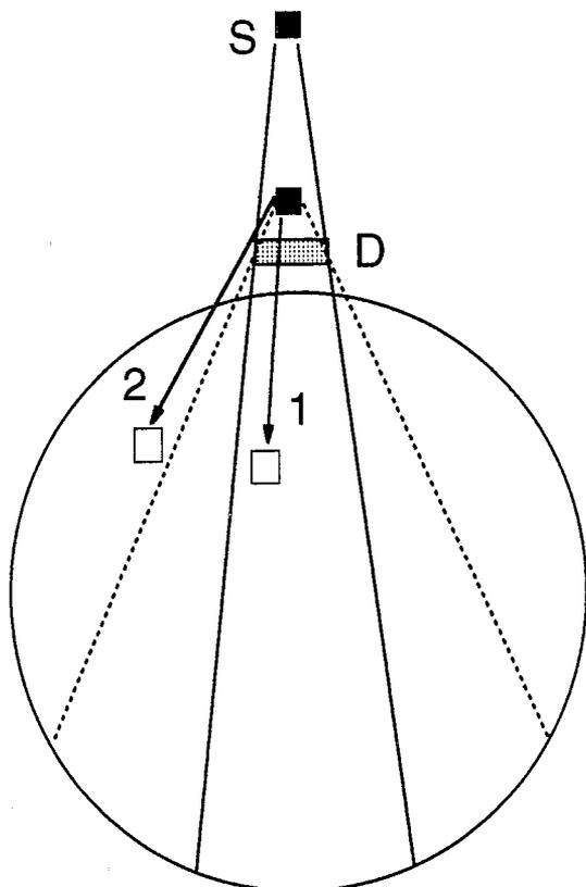
Fig. 1. Diagram showing the decrease of volume and mass of the Earth which can be shielded in principle by the disc (D), as a function of the distance of the sample (S) above the disc. See text for details.
