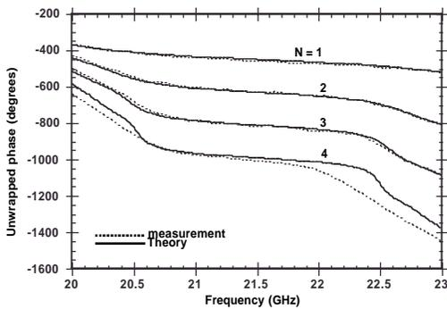
**Fig 5:** The unwrapped transmission phase for the 1DPC with various number of Eccostock<sup>®</sup> dielectric slabs.
