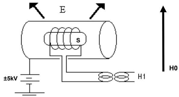
Figure 1. NMR "can" arrangement. External magnetic field, H<sub>0</sub>, is perpendicular to the radio frequency field, H<sub>1</sub>, applied through a coil wrapped around the proton sample, S. The 5kV electric field is applied outside the can leaving a constant 5kV potential inside.
