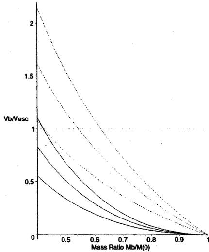
Figure 2: These plots indicate the mass ratio  $M(t_b)/M(0)$  required to reach a non-relativistic speed  $V_b$  in the presence of the earth's (uniform) gravitational field.  $V_{esc}$  is the escape velocity for the earth. The upper three (dotted) curves correspond to a specific thrust parameter  $\mathcal{R} = 2$ . The lower three (full) curves correspond to  $\mathcal{R} = 1$ . In each triplet the ejection speed is chosen to vary according to three typical chemical propellants.
